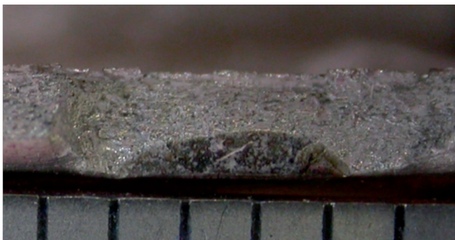
Figure 2 Destructive examination results for axial cracks in austenitic stainless steel steam generator tubes.
