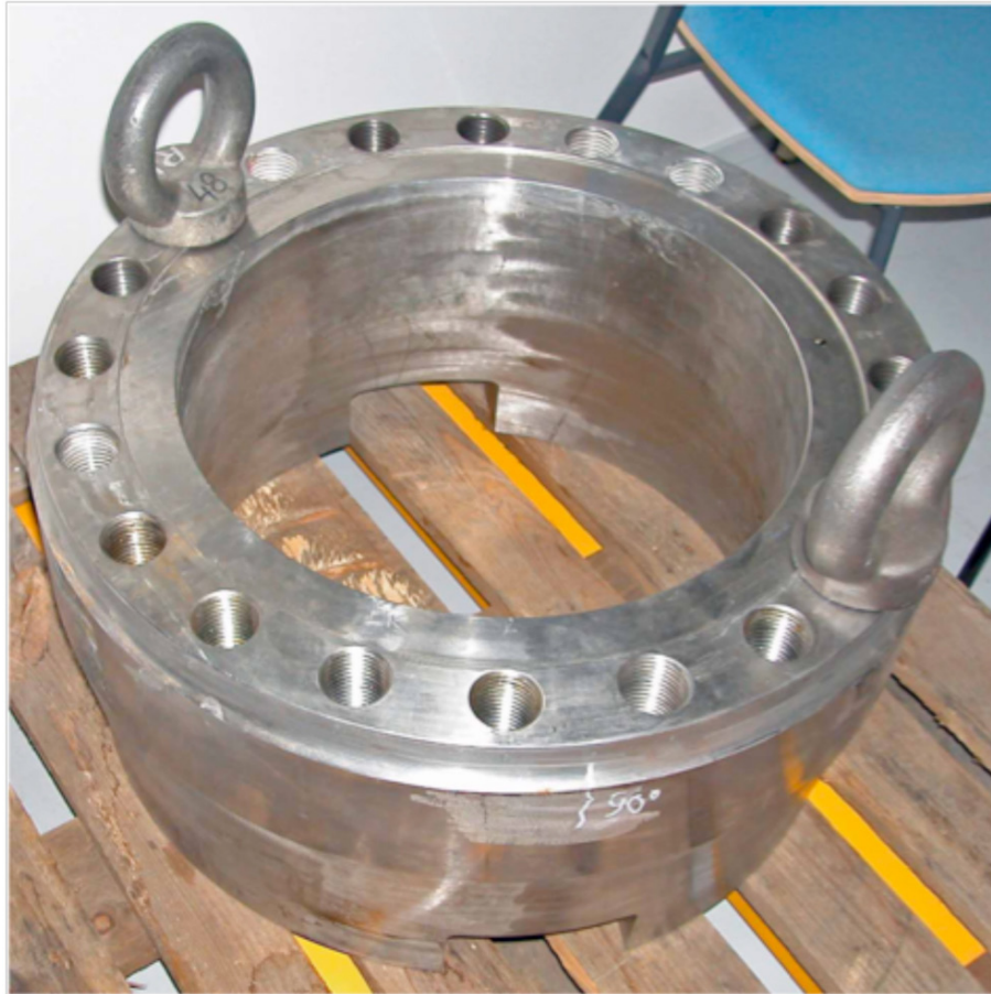
Figure 2 Loviisa test block from vintage material.
